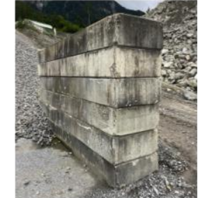
Crane counterweights 430 x 80 x 35 cm – 14 pcs. partially cut, upright
