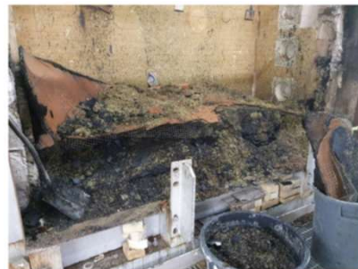
Plaster system collapsed when extinguishing the test specimen
