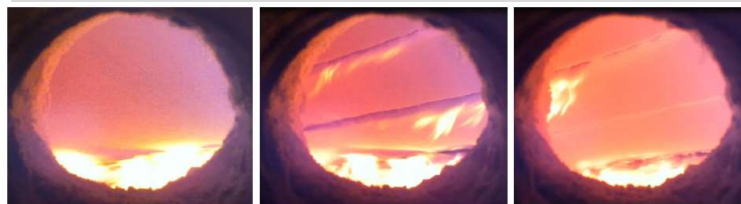
First crack 19 min Largest cracks 31 min Before fall-off 75 min
